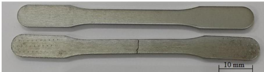
**Fig. 2.** General view before and after tensile tests specimen obtained from Alloy 2 sintered at 1400°C.
