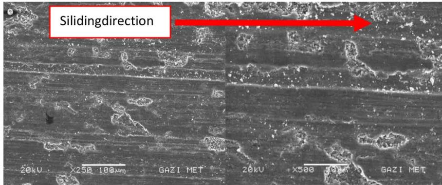
**Fig. 9.** SEM images of AA 7075 aluminum after wear.
