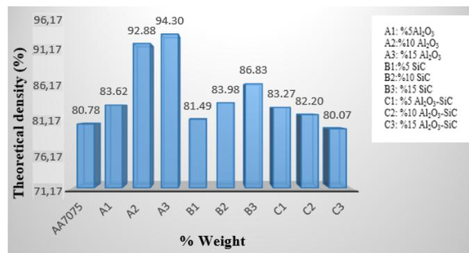
**Fig. 2.** Density values of hybrid/composite samples according to % particle rate of samples after sintering.
