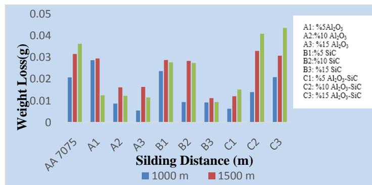
**Fig. 8.** Weight loss of test samples after wear.
