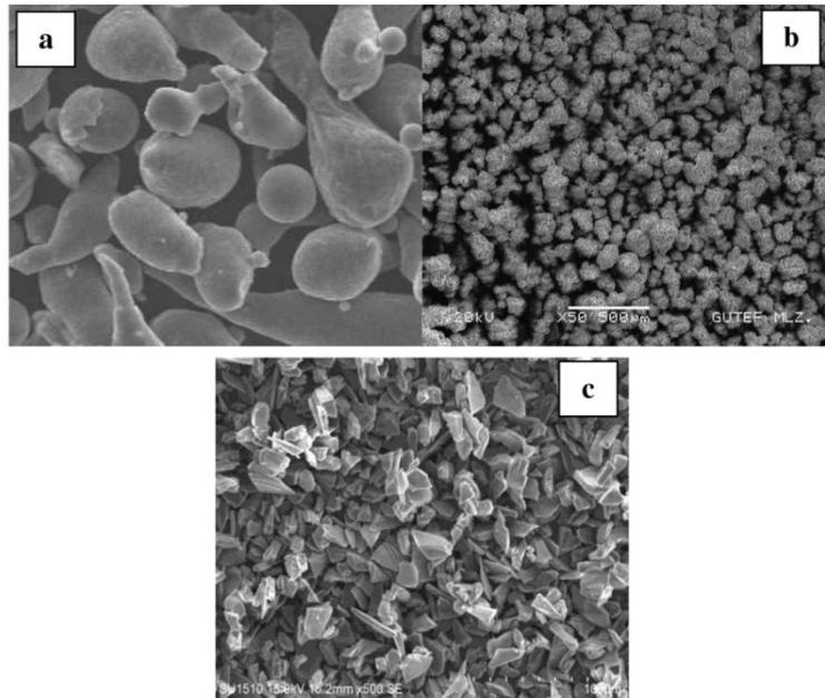
**Fig. 1.** SEM images of starting powder materials; a) AA7075, b)  $\text{Al}_2\text{O}_3$ , c) SiC.
