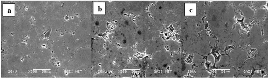
**Fig. 5.** SEM images of composite samples after sintering: a) %5SiC, b) %10SiC, c) %15SiC.
