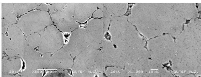
**Fig. 3.** After sintering AA7075 aluminum material SEM images.
