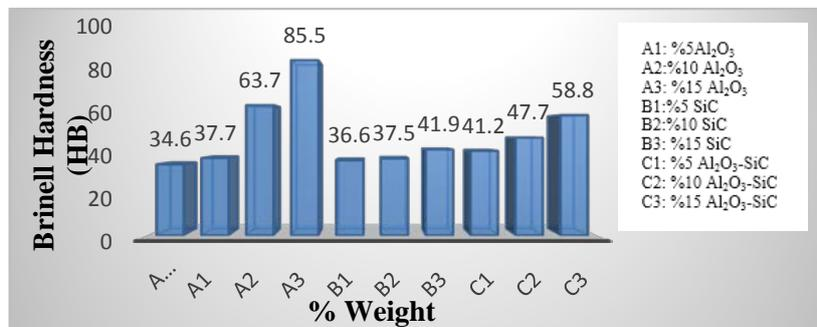
**Fig. 7.** Hardness results of test samples after sintering.
