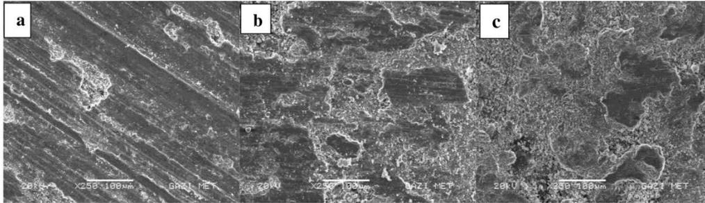
**Fig. 12.** SEM images of AA7075 +  $\text{Al}_2\text{O}_3$ -SiC wear surface: a) %5 b) %10, c) %15.
