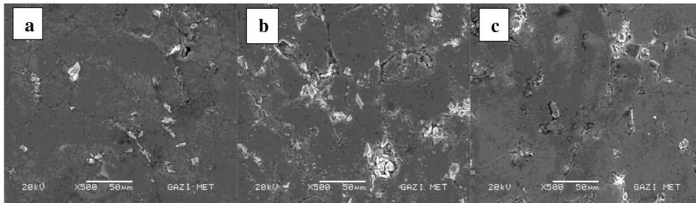
**Fig. 6.** SEM images of hybrid composite samples after sintering: a) %5 Al<sub>2</sub>O<sub>3</sub>-SiC, b) %10 Al<sub>2</sub>O<sub>3</sub>-SiC, c) %15 Al<sub>2</sub>O<sub>3</sub>-SiC.
