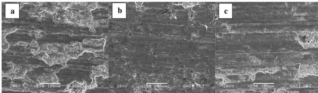
**Fig. 11.** SEM images of AA7075 + SiC wear surface: a) %5 b) %10, c) %15.
