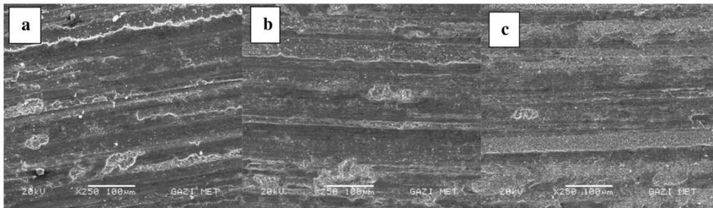
**Fig. 10.** SEM images of AA7075 + Al<sub>2</sub>O<sub>3</sub> wear surface: a) %5 b) %10, c) %15.
