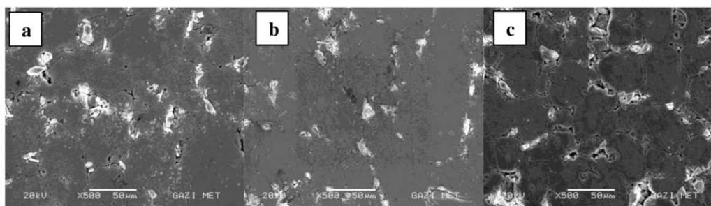
**Fig. 4.** SEM images of composite samples after sintering: a) %5 $\text{Al}_2\text{O}_3$ , b) %10 $\text{Al}_2\text{O}_3$ , c) %15 $\text{Al}_2\text{O}_3$ .
